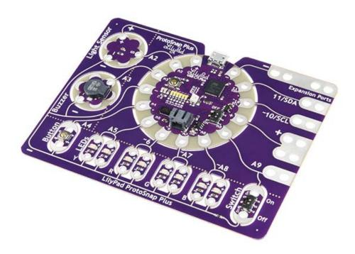
The LilyPad ProtoSnap Plus is a sewable electronics prototyping board that you can use to explore circuits and programming, then break apart to make an interactive fabric or wearable project. Programming the ProtoSnap Plus is easy with the free Arduino software you'll need to program the ATmega32U4 on LilyPad USB Plus at the heart of the board. Once you've installed the software, you'll be able to write and upload your own programs to the board, making it do almost anything you want.
