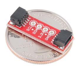
The SparkFun Qwiic Adapter provides the perfect means to make any old I<sup>2</sup>C board into a Qwiic-enabled board. This adapter breaks out the I<sup>2</sup>C pins from the Qwiic connectors to pins that you can easily solder with your favorite I<sup>2</sup>C-enabled device.
