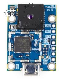
**LED:** When plugged in to micro-usb power and a Lepton is inserted in the socket LED will flash slowly. When video is being transmitted to the viewing program, LED will flash more rapidly.
