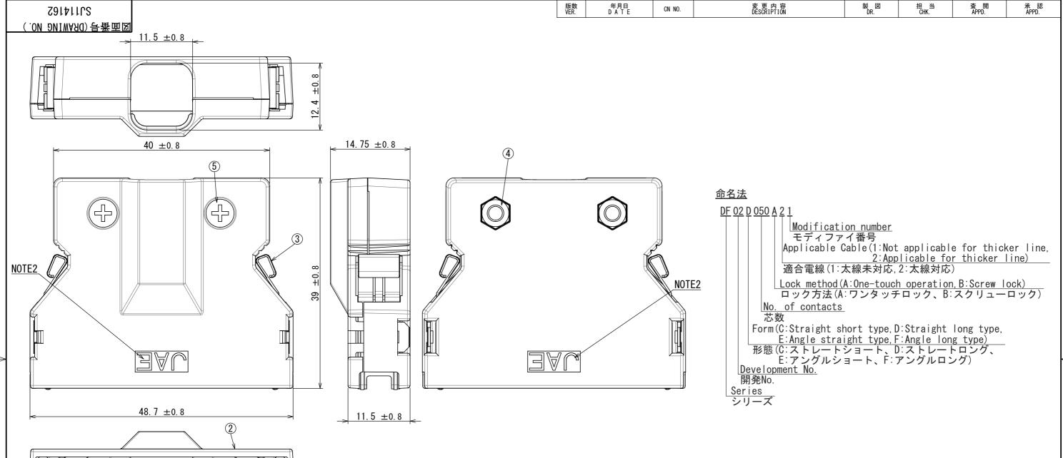
NOTE1. THE HOOD (A) ASSEMBLED WITH NUT IS SUPPLIED. THE OTHER PARTS ARE ATTACHED.
