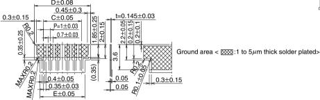
Signal area < 8883:1 to  $5\mu$ m thick solder plated>
