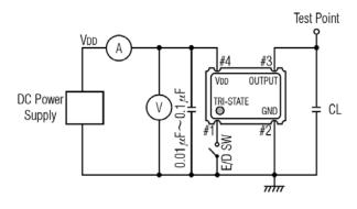
Figure 1) Test Circuit
