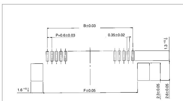
**DF21 Series 0.6mm Pitch Board-to-Fine Coaxial Cable Connectors**
