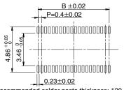
Recommended solder paste thickness: 120  $\mu$ m
