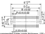
Recommended solder paste thickness: 120  $\mu$ m
