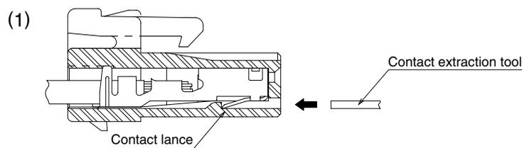
1. Refer to the drawing No. 1. Insert contact extraction tool in the insulator against the lance. Deflect the lance as shown.
