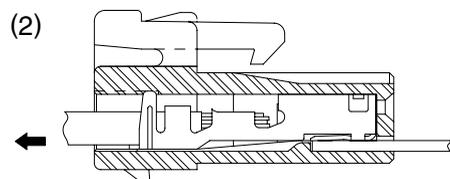
2. Assure that the lance is deflected to release the contact and pull- out wire with the terminated contact.
