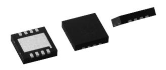
The DFN series of precision surface mount resistor networks feature isolated thin film precision resistors mounted in a 0.8 mm pitch 4 mm x 4 mm dual flat no lead package. The networks feature 50 % savings in board space over traditional SOIC packages. They are ideally suited for applications of unity gain operational amplifiers that require close TC tracking and tight ratio tolerances over temperature. Custom configurations are available upon request.
