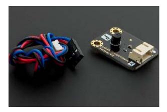
DFRobot LM35 Linear Temperature Sensor
