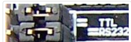
(/wiki/index.php/File:Sdb_v2.2_5.pr RS232/TTL Selection Jumpers
