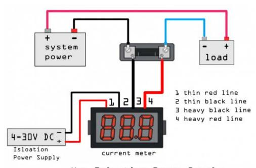
Use Isloation Power Supply Connection Diagram
