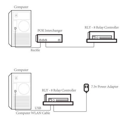
**NOTE**: If you choose directly connect to the computer. Then the computer have to be set to a fixed IP, you can set computer's IP as 192.168.1.8, netmask 255.255.255.0, gateway 192.168.1.1
