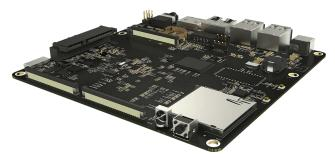
LOFT-Q is the second series prototyping board of Mixtle Project. Based on Allwinner A31 soc, This board is well designed for embedded developers and engineers, makers and geekers, which could be used as Home Media Center, personal cloud platform, NAS, etc.
