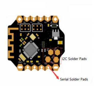
• 2. When soldering the Beetle to the Shield, make sure the orientation of the Beetle is correct so as to avoid connecting the wrong pins. The beetle should sit on the shield as pictured:
