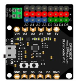
• 3. Please note that the Vcc pins for analog expansion pins is fixed at 5v. The Vcc pins for digital expansion pins is dependent on your power supply (5-8v DC)
