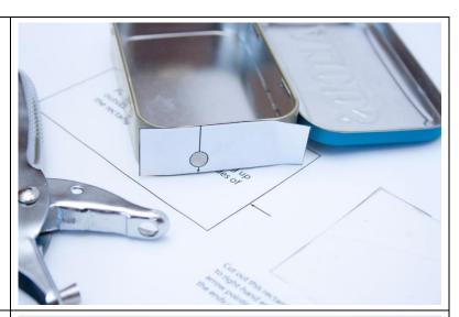
Next, cut out the rectangle on the lower half of the page and glue it onto the colored side of a sheet of thin cardboard (cereal-box cardboard, etc.). Then cut it out on the outline. The cardboard will serve to insulate the bottom of the PCB from the tin.
