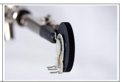
Now insert the first wheel into the PCB as shown.
