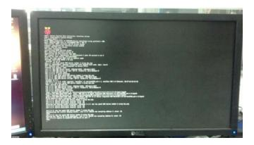
2. The flow of text will stop at the user login screen. Enter user name: "pi", password: "raspberry"
