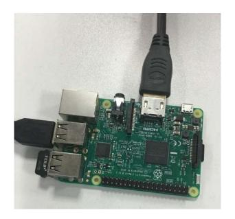
9. Connect the USB power cord and turn on the power
