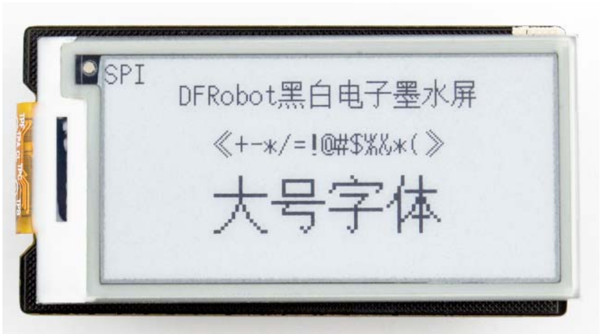
FireBeetle Covers-ePaper Black&White Display Module(SPI)
