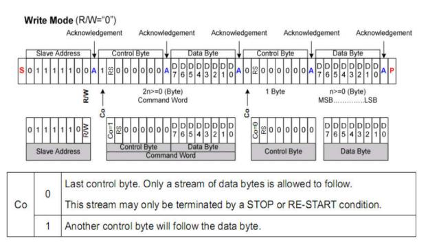
AiP31068L (LCD ) Slave Address : 0X7C. PCA9633DP2 (RGB) Slave Address: 0XC0.
