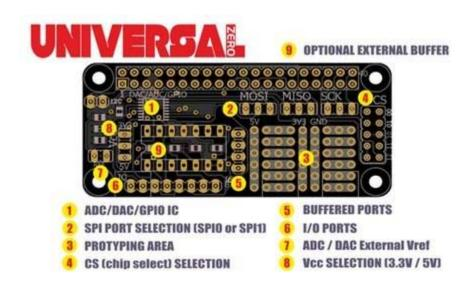
The board's ADC/DAC/GPIO IC can be supplied from 5V (jumper 8). It gives a potential possibility to measure directly voltages up to 5V (up to Vcc actually). This is an experimental feature, and it is very probable to damage your PI if the 5V option is used. Please always use 3.3V option.
