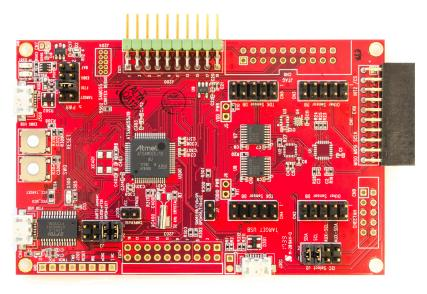
The development kit comes with necessary software including InvenSense MotionLink, a GUI based development tool and embedded Motion Drivers for ICP-10100.
