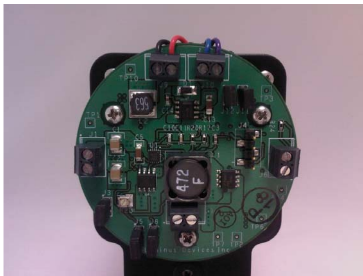
Figure 5: Completed electrical connections on DK-105T-1
