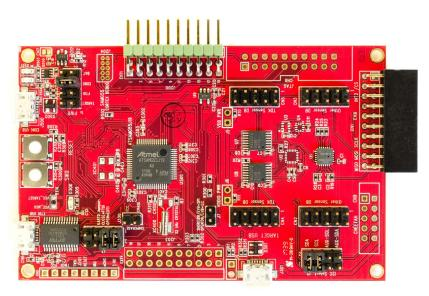
The development kit comes with necessary software including InvenSense MotionLink, a GUI based development tool and embedded Motion Drivers for ICM-20789.
