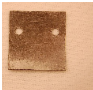
Figure 2: TIM cut for CBM and CSM package types.
