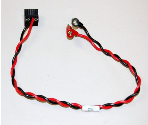
Figure 3: Power supply to driver board cable
