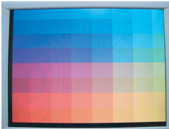
Figure 2–3. Default FGA Output Pattern, SW0 = UP
