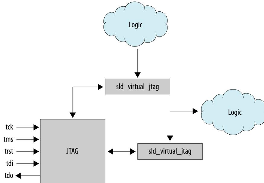
The hub automatically arbitrates between multiple applications that share a single JTAG resource. Therefore, you can use the IP core in tandem with other on-chip debugging applications, such as the Signal Tap logic analyzer, to increase debugging visibility. You can also use the IP core to provide simple stimulus patterns to solicit a response from the design under test during run-time, including the following applications:
