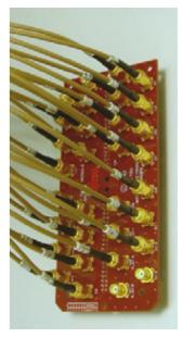
Adaptors provide a convenient conversion from SMA to the Motherboard's 0.1" headers. This simplifies the simultaneous removal of 28 SMAs (14-bit differential LVDS) when required. One advantage of this is the ability to swap the data generator easily between DAC data ports if insufficient channels are available to drive both ports simultaneously.
