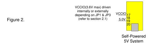
Figure 2 illustrates a typical USB self-powered configuration. A USB self-powered device gets its power from its own power supply and does not draw current from the USB bus.
