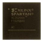
The FPGA device used on the DLP-HS-FPGA is the Xilinx Spartan<sup>™</sup> 3A: XC3S200A-4FTG256
