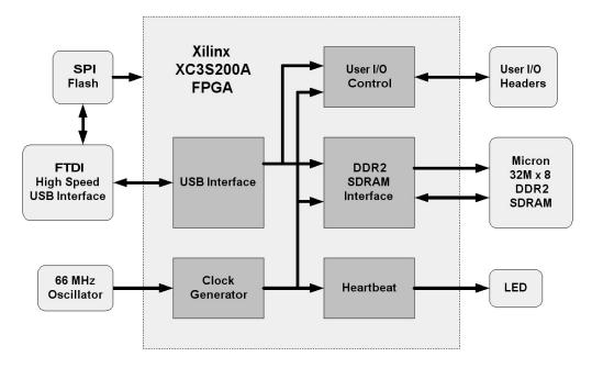
It contains a USB interface block, a User I/0 block, a DDR2 SDRAM interface, a Heartbeat pulse generator, and a clock generator. The SPI Flash is used to store the design's FPGA configuration file.
