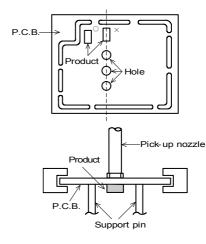
P.C.B. shall not be separated with hand. P.C.B. shall be separated with the fixture so as not to cause P.C.B. bending.
