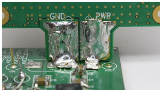
Figure 1. DLT Attached with Solder Wick
