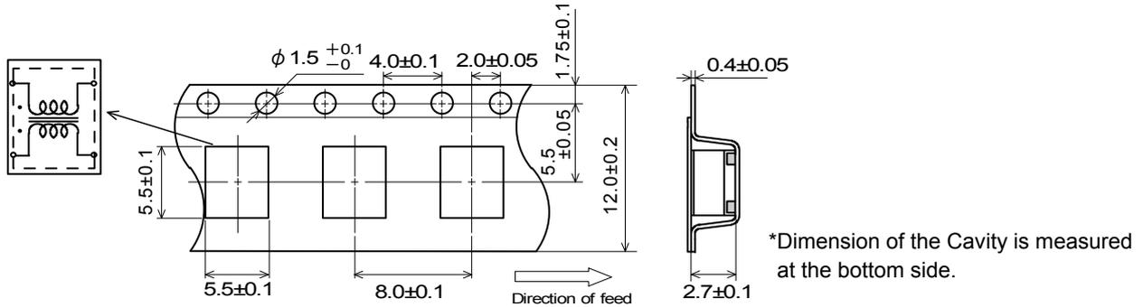
\*Dimension of the Cavity is measured at the bottom side.
