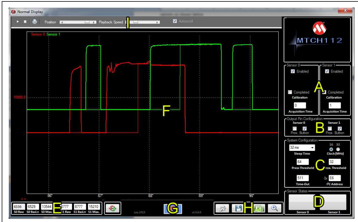
FIGURE 1-7: MTCH112 GUI FUNCTIONAL AREAS
