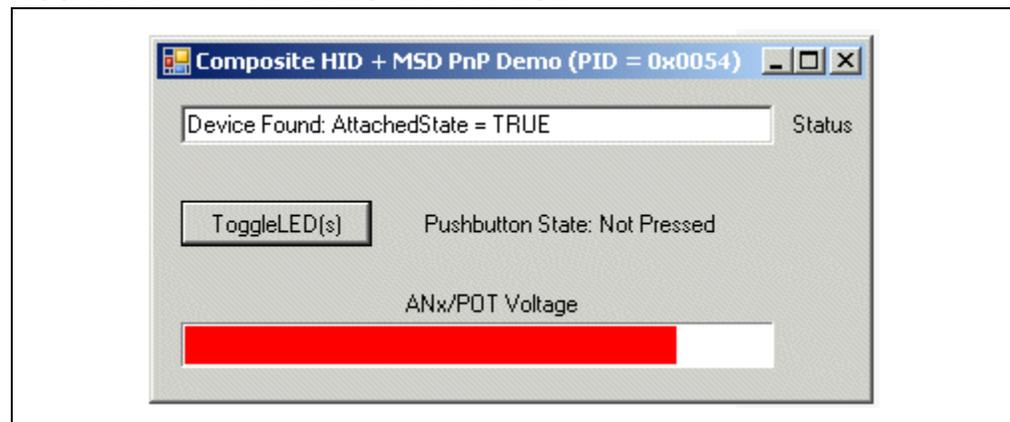
The demo PC application provides a simple graphical user interface for sending and receiving small amounts of example data to and from the HID interface on the USB device. Full source code for both this PC application and the demo firmware are
