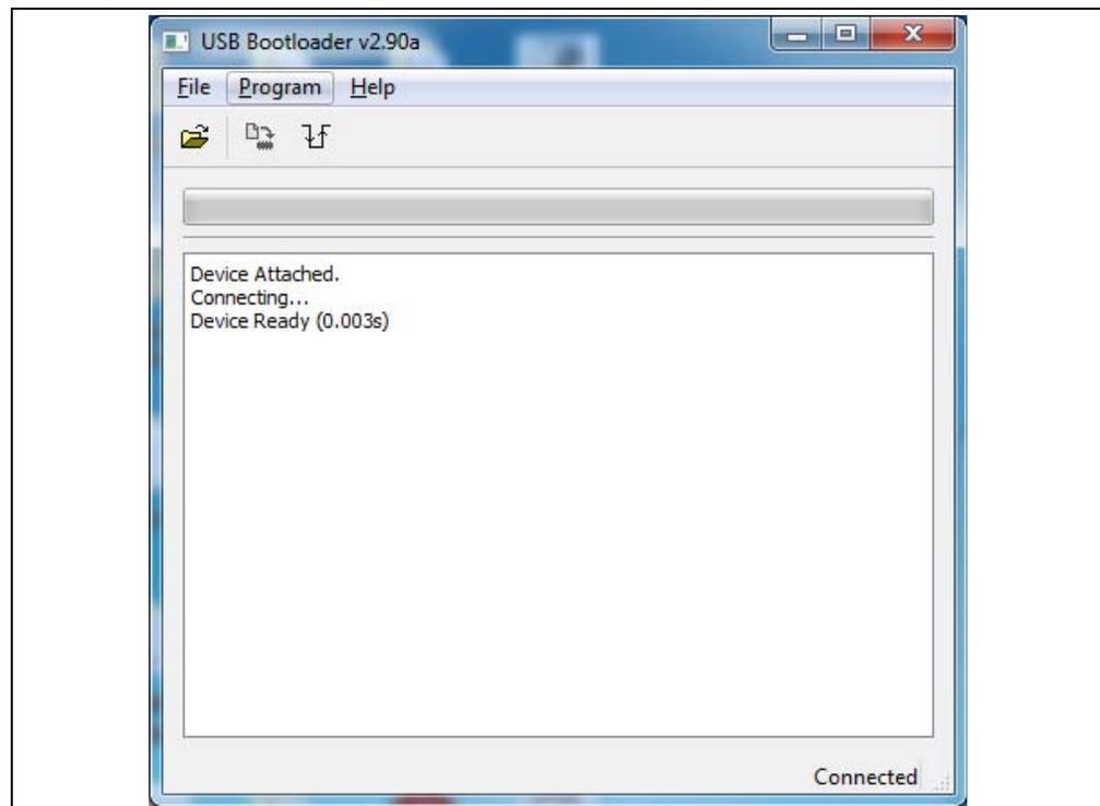
Once the PC application has found the USB device, the application can be used to open the Intel® HEX 32-bit formatted \* .hex firmware images and program them using the respective buttons.
