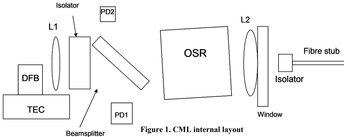
Figure 1. CML internal layout
