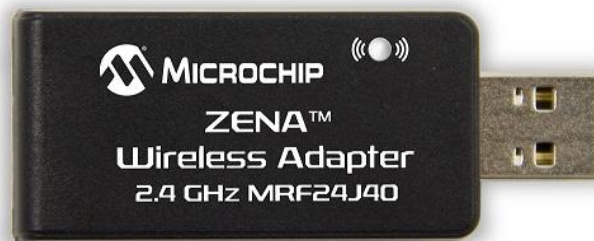
ZENA™ Wireless Adapter – 2.4 GHz MRF24J40 (Part # AC182015-1)
