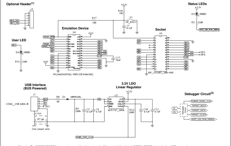
**Note 1:** The PGEC2/PGED2 pins can be used for debugging via J3 instead of the default PGEC1/PGED1 pins via the USB connection.
