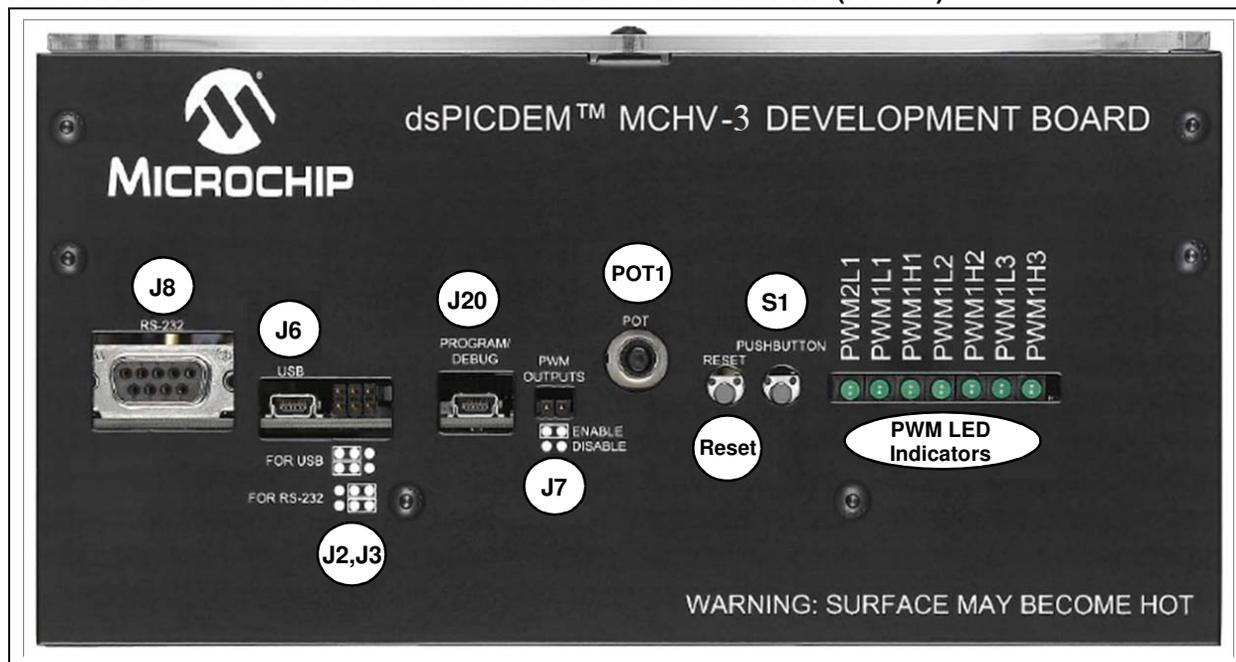
**FIGURE 2-3: dsPICDEM™ MCHV-3 DEVELOPMENT BOARD (LEFT SIDE)**
