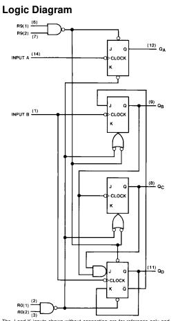
The J and K inputs shown without connection are for reference only and are functionally at a HIGH level.
