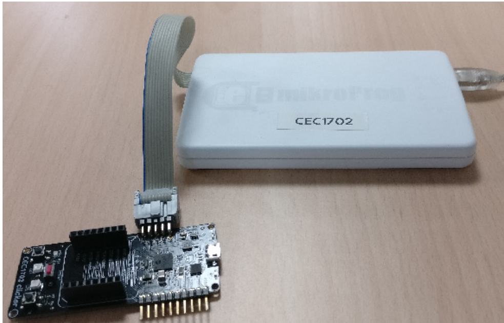
FIGURE B-1: CEC1702 CLICKER BOARD SETUP
