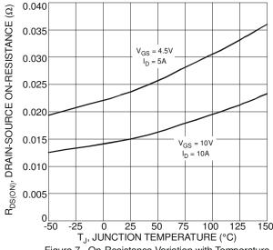
Figure 7. On-Resistance Variation with Temperature
