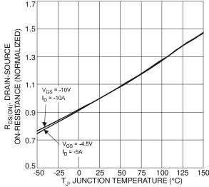
Figure 18. On-Resistance Variation with Temperature
