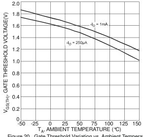
Figure 20. Gate Threshold Variation vs. Ambient Temperature
