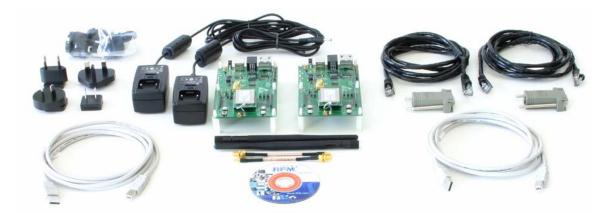
900 MHz Frequency Hopping Transceiver Module Development Kit
