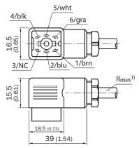
Minimum bend radius at dynamic use  $R_{Min}$  = 20 x cable diameter
