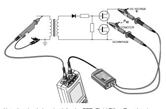
Note that the timing circuit for the FET (Field Effect Transistor) drive is referenced to earth ground. The gate drive signal is isolated with a transformer coupling to the FET, which is connected to the
