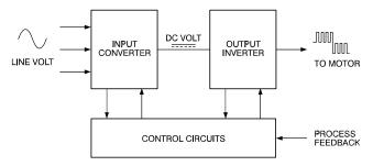
When one of the stages of the output inverter does not function properly, check the following:
