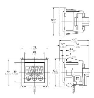
portion shows the front protection cover. Material: Polycarbonate (Front protection cover)
