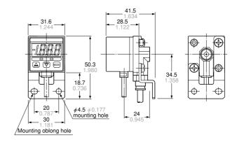
Material: Cold rolled carbon steel (SPCC) (Uni-chrome plated)
