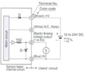
Note: In case the pressure sensor head is used independently, insulate the white wire (Terminal No.4) and keep it open.
