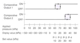
Note: In the hysteresis mode the displayed values and the ON/OFF points of the output are changed in case the output mode is set to the window comparator mode. Remote zero-adjustment input: 50kPa
