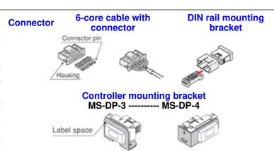
You can attach a commercially available label (9 mm) to the top of the unit to display the sensor number and the sensor application.
