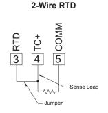
CAUTION: Sensor input common is NOT isolated from user input common. In order to preserve the safety of the meter application, the sensor input common must be suitably isolated from hazardous live earth referenced voltages; or input common must be at protective earth ground potential. If not, hazardous live voltage may be present at the User Input and User Input Common terminals. Appropriate considerations must then be given to the potential of the user input common with
