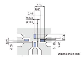
Line width should be designed to match  $50\Omega$  characteristic impedance, depending on PCB material and thickness.
